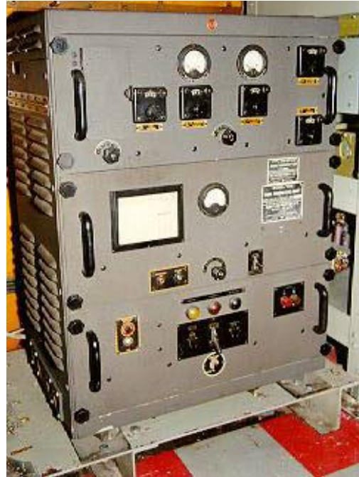
Figure 9-23 TDQ (CRV 52328) VHF Transmitter. The TDQ can transmit about 45 watts of CW, MCW, or Voice on frequencies ranging from 115 to 156mc. Output is limited to four channels at-a-time and is controlled by crystals in a temperature-controlled oven that kept them at a constant 70 degrees Celsius. The transmitter is 32" tall, 25" wide, and weighs 283 lbs. Aboard ship it was typically controlled remotely by a radiophone unit (shown below).
