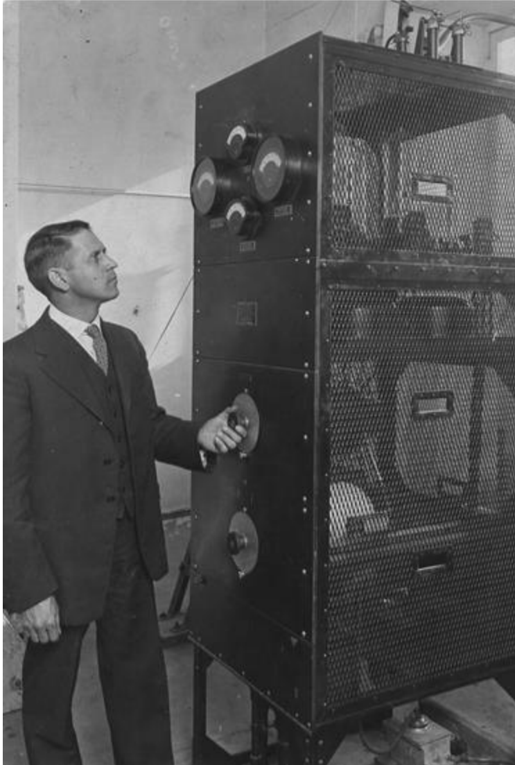
Figure 4-18 KGW's Western Electric Model 1-B AM transmitter (date unknown). KGW installed this 1 kw transmitter at their downtown station in 1926 and moved it to Vanport in 1931. (Oregonian files from KGW AINW report)
