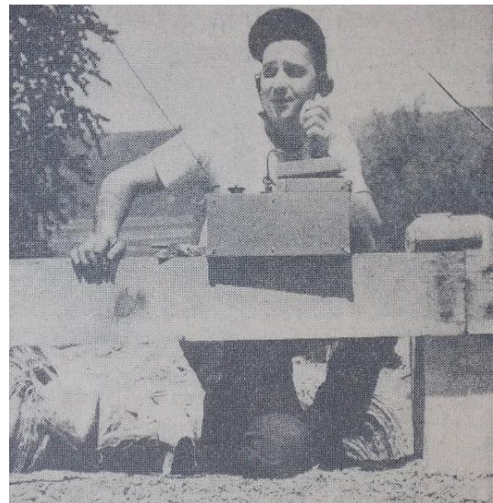
Figure 7-11 Eldon Stevens keeps watch on a dike near Blue Lake. He's using a Forest Service Type SX 30-40 mc transceiver. (The Oregonian 6/3/48)
